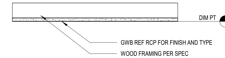
TYPICAL GWB C2 | CEILING HEIGHT NOTED A.F.F.
